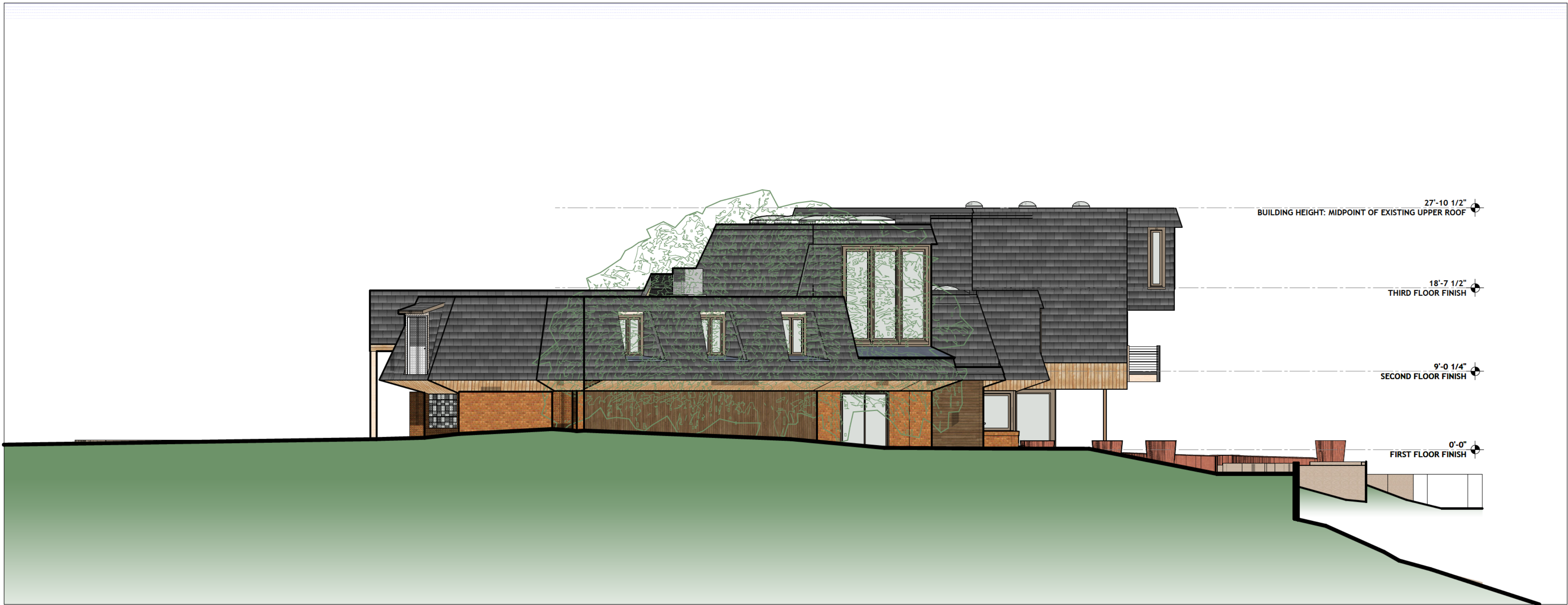
2 WEST EXTERIOR ELEVATION (EXISTING) 1/8" = 1'-0"
