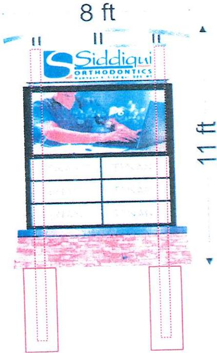
4" x 4" x 0.25" wall, A500 46ksi HSS Steel Column, S=3.9 IN<sup>4</sup>
