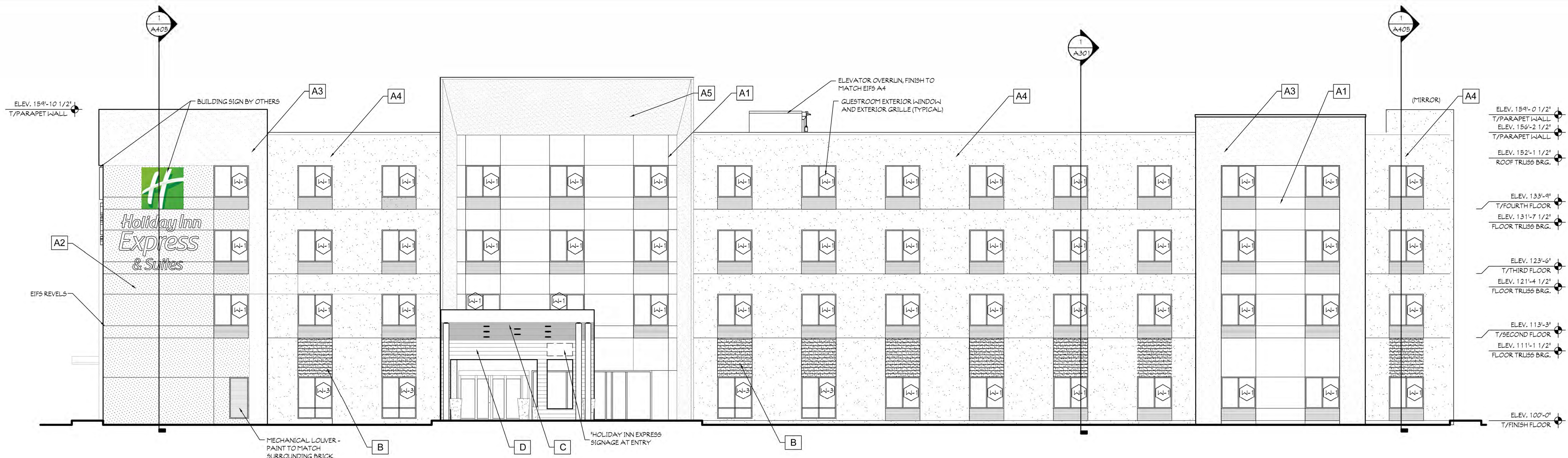
1 EXTERIOR ELEVATION SCALE: 1/8" = 1'-0" NORTH (FRONT) ELEVATION
