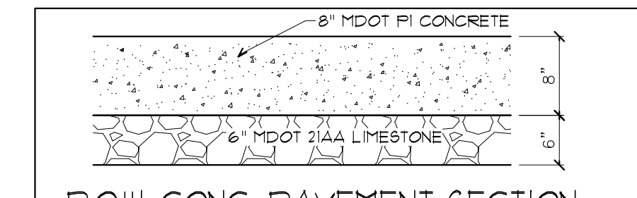
R.O.W. CONC. PAVEMENT SECTION
