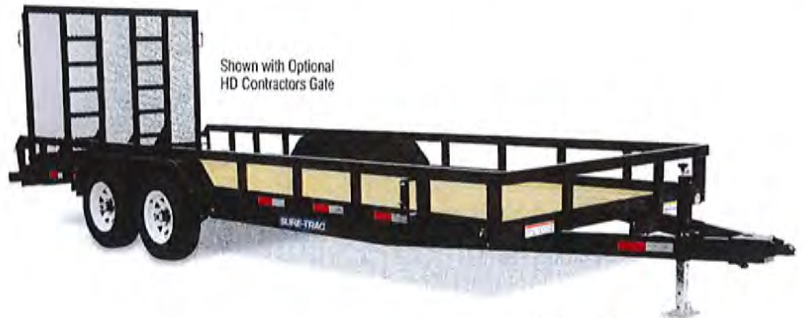
10K Model Features 7k Dropleg Jack, 3 x 2 Tube Top Rail and Reinforced Gate
