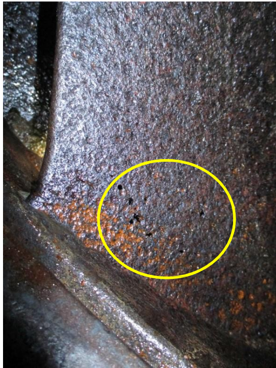
Runner- Showing pin holes that are forming
