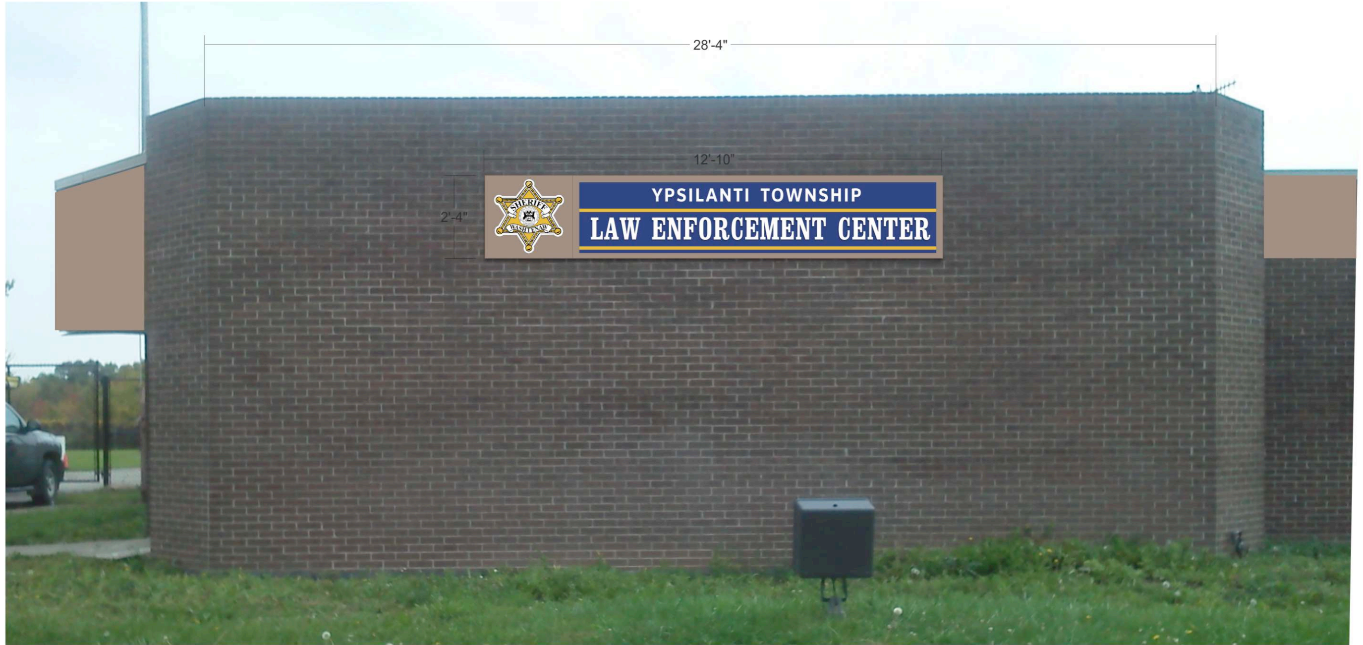
NEW 1 1/2" DEEP ALUMINUM PAN WALL SIGN WITH BLIND INSTALLATION BRACKET AND APPLIED VINYL GRAPHICS. OPTIONAL RAISED LETTERS
