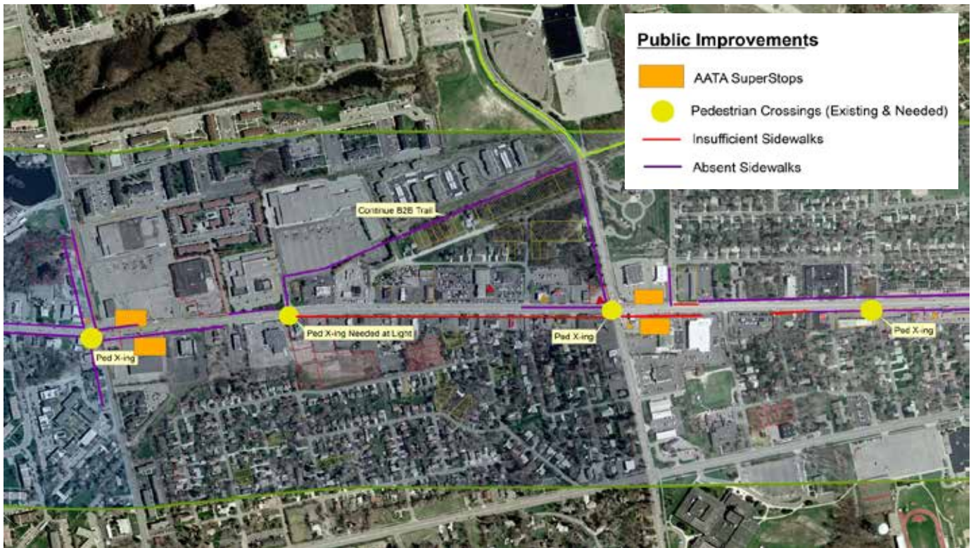
A map prepared as part of Washtenaw County's ReImagine Washtenaw project shows sidewalk gaps along Washtenaw Avenue in the Township
