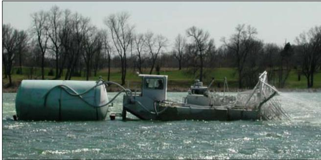
Barr worked with the Sauk River Watershed District on an alum treatment project to improve the water quality of Lake Osakis by reducing phosphorus inputs from sediment in the Faille Chain of Lakes. We collected sediment core samples from the three lakes, extruded and sectioned them, and sent them out for analyses of iron-bound and labile-phosphorus fractions. Based on the results of these analyses, we calculated alum dose rates and specified the treatment regimen for the
