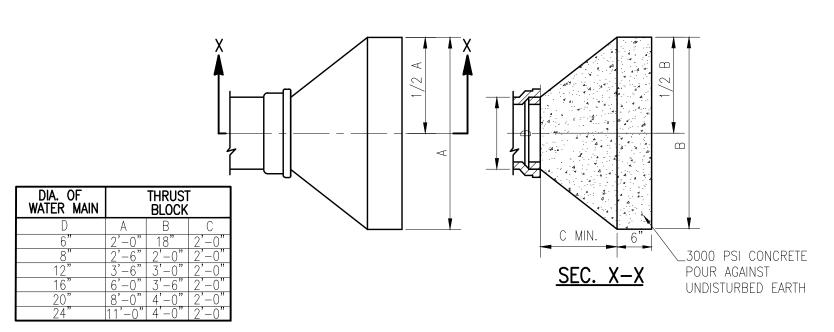
THRUST BLOCK AT PLUG OR HYDRANT SHOE
