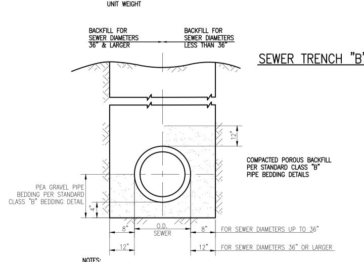
1. SUITABLE EXCAVATED BACKFILL MATERIAL SHALL BE PLACED IN ONE FOOT LAYERS AND COMPACTED BY MECHANICAL TAMPING OR OTHER EFFECTIVE MEANS HAVING APPROVAL OF THE ENGINEER. TO A DENSITY EQUIVALENT TO THE UNDISTURBED ADJACENT SOIL 2. TRENCH "B" SHALL BE USED UNDER CONDITIONS
