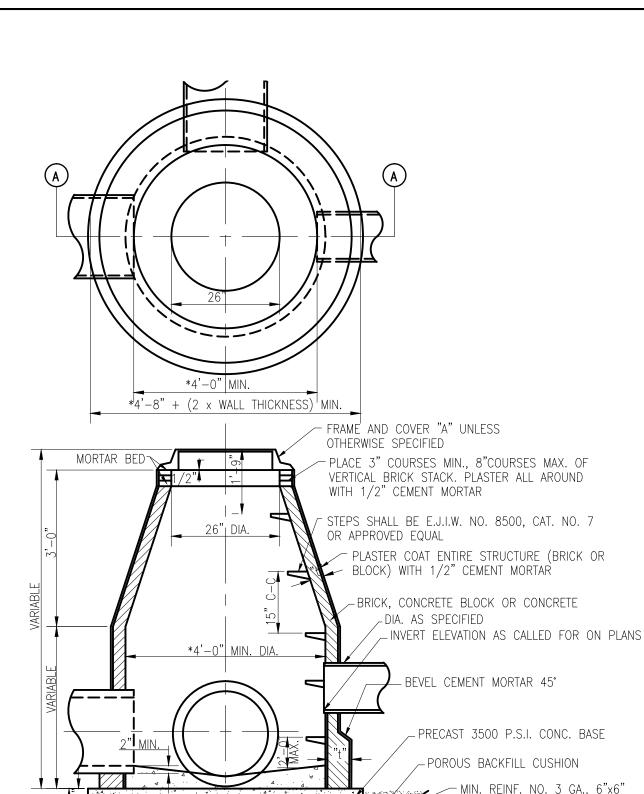
1. MANHOLE "B" SHALL BE USED FOR MANHOLE STRUCTURES ON ALL STORM SEWERS WHERE THE DIAMETER OF OUTLET PIPE IS 24" OR SMALLER, UNLESS CALLED FOR OTHERWISE ON THE PLANS.
