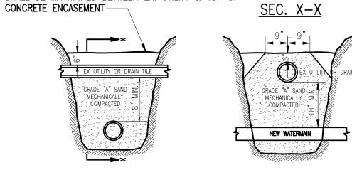
COMPACTED SAND SHALL EXTEND FOR 9" EACH SIDE OF EXISTING PIPE, AT 6" ABOVE EXISTING PIPE & SHALL SLOPE OUT AT A 1:1 (45°) SLOPE TO THE BOTTOM OF THE TRENCH
