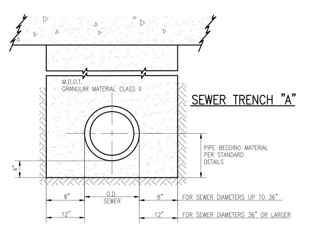
1. TRENCH "A" SHALL BE USED UNDER ROAD SURFACES, PAVEMENT, SIDEWALK, CURB, AGGREGATE & PAVED DRIVES AND WHERE THE EDGE OF TRENCH IS WITHIN 3 FEET OF THE PAVEMENT
