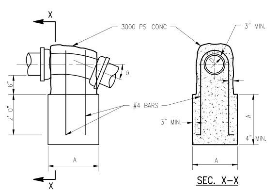
DETAIL OF VERTICAL ANCHORAGE NOT TO SCALE
