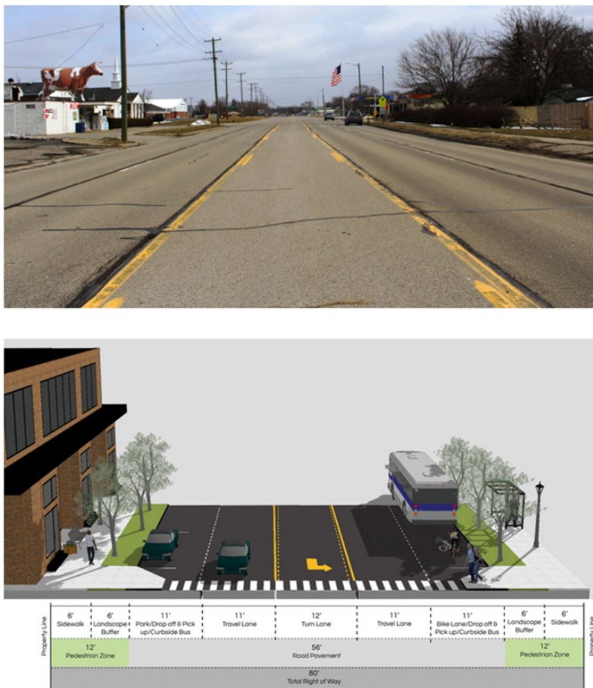
Figure 6: Existing Conditions (top image) versus Illustrative Road Diet with Mixed-Use Pedestrian-Oriented Development (bottom)
